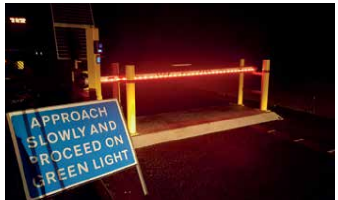
ABOVE: SOSEC barriers can operate up to 900 times a day.
