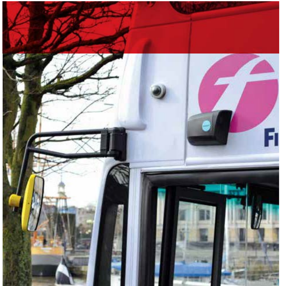
RIGHT: First buses in Bristol has been trialing a cyclist detection and alert system which uses radar and vision technologies.
